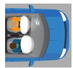
A "deployment event" is recorded onto the black box when it detected higher than normal accelerations and sent a signal for the airbags to deploy during a collision.
